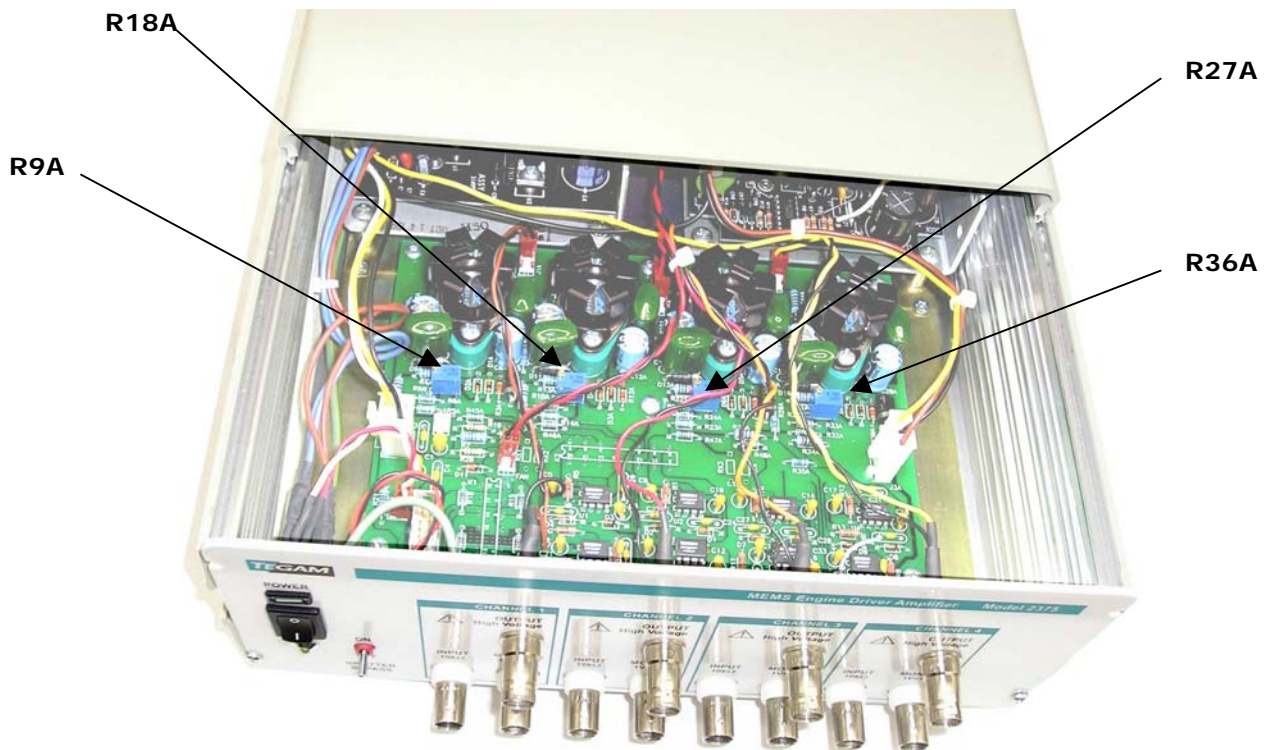
Figure 5: – Power Amplifier Gain/Offset Adjustments
